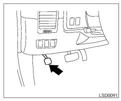
**To engage:** Firmly depress the parking brake.
