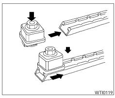
They must be installed so they are properly seated in the detents in the channel.
