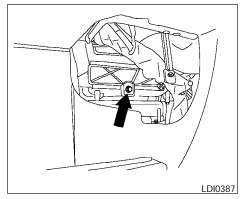
3. Remove the filter cover bolt and remove the filter cover.
