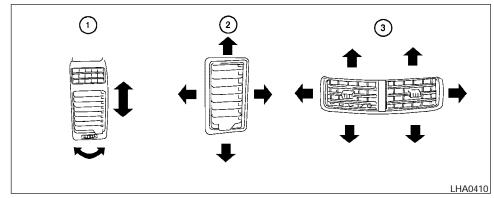
Adjust air flow direction for the driver and passenger side 1, center 2, and rear passenger (if so equipped) (3) ventilators by moving the ventilator slide and/or ventilator assemblies.
