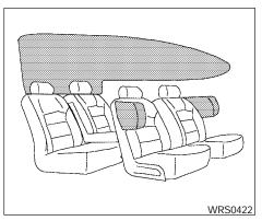
Supplemental side-impact air bag (if so equipped) and curtain side-impact and rollover air bags system
