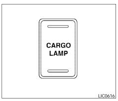
To turn on the cargo lamp, push the switch down to the ON position. The tailgate lights (if so equipped) will also illuminate when the cargo lamp switch is in the ON position.
