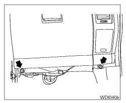
1. Remove the two lower glove box screws.
