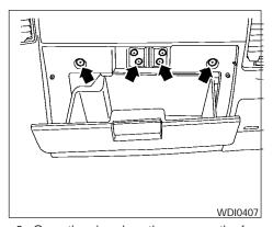
2. Open the glove box, then remove the four upper glove box screw. It is not necessary to remove the two glove box striker screws. Remove the glove box assembly from the instrument panel to access the in-cabin mi-
