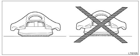
There should be no gap between the bottom of the cleat and the top of the channel. Tighten the center bolt hand tight (20-40 inch pounds).
