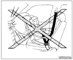
Even with the NISSAN Advanced Air Bag System, never install a rear-facing child restraint in the front seat. An inflating supplemental front air bag could seriously injure or kill your child. See "Child restraints" later in this section for details.
