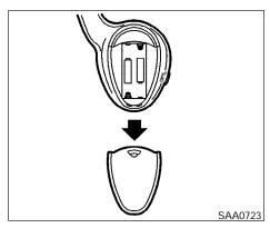
If the battery is removed for any reason other than replacement close the lid securely.
