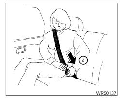
Slowly pull the seat belt out of the retractor and insert the tongue into the buckle until you hear and feel the latch engage.
