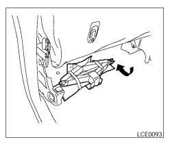
2. Unscrew and remove the jack and tool kit.
